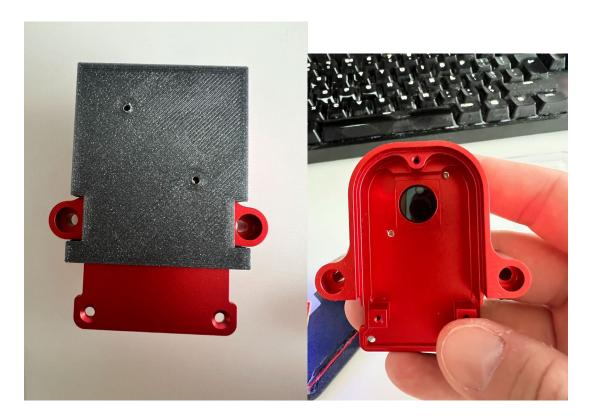
The recommended way would be to remove the PCB and silicone seal, but, if you can drill the holes to be 2-3mm, you can jump straight to step #3 in the guide
