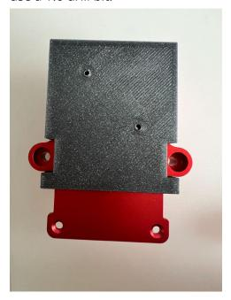
Fit the lens into the mount and put everything in place using the M2 screws provided.
