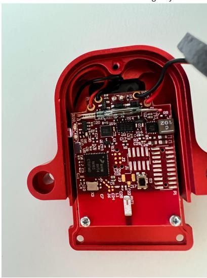
Remove the two screws that fix the PCB to the case and gently push the camera and silicone seal out
