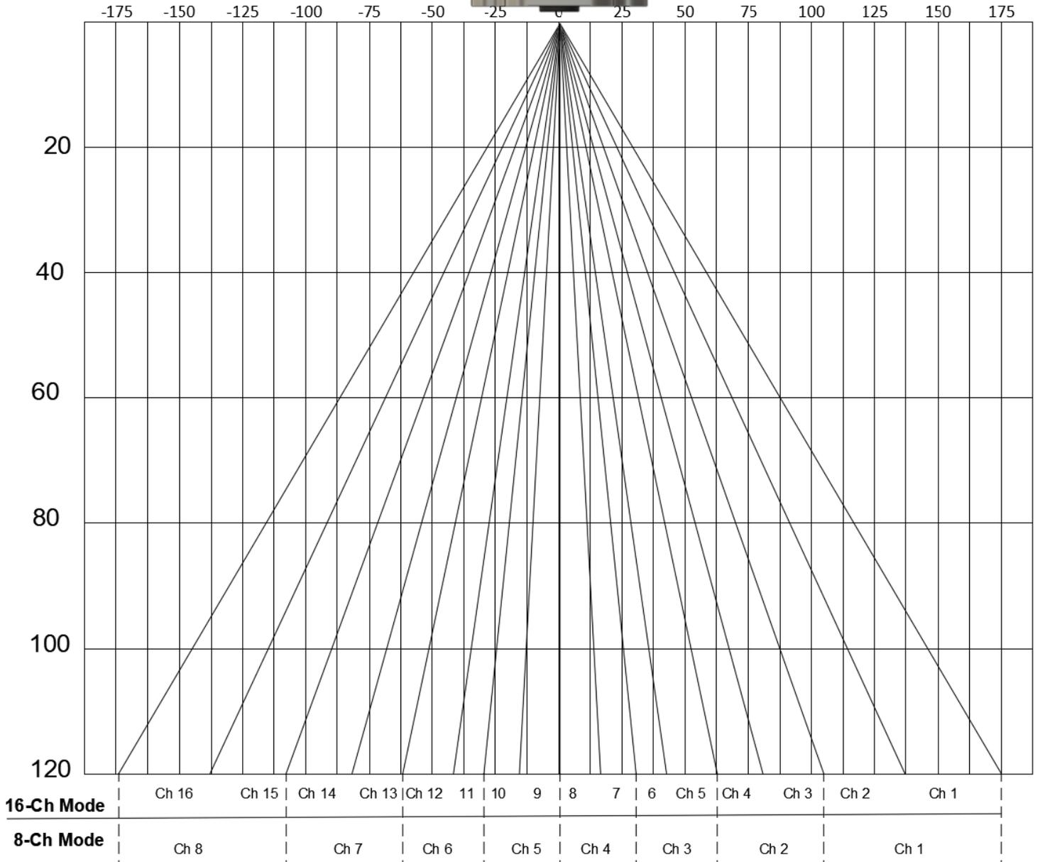
Figure 2 - Visual Representation of channel assignments
